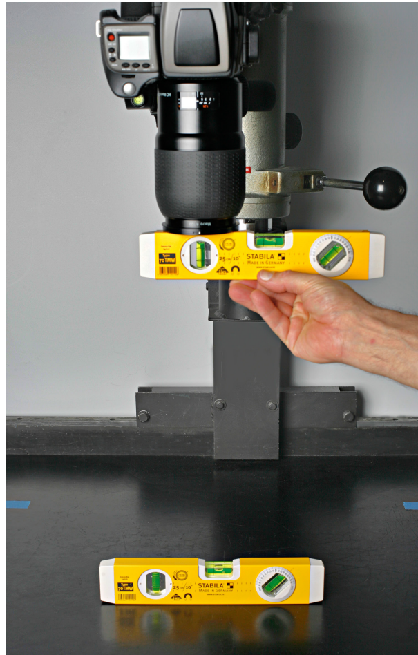
Aligning the yaw of a DSLR lens relative to the baseboard
